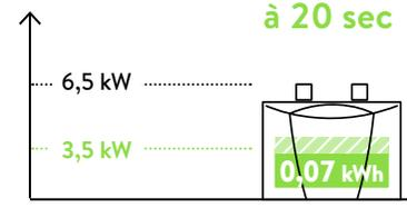
$2 \text{ l/min} \times 0,33 \text{ min} \times 4/\text{d} \times 1,163 \times 23\text{K} = 71 \text{ Wh} = \mathbf{0,07 \text{ kWh}}$
