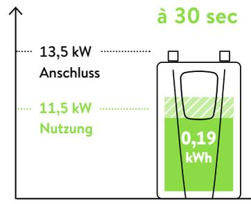
$5 \text{ l/min} \times 0,5 \text{ min} \times 2/\text{d} \times 1,163 \times 33\text{K} = 191 \text{ Wh} = \mathbf{0,19 \text{ kWh}}$
