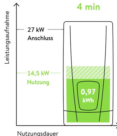
$8 \text{ l/min} \times 4 \text{ min} \times 1,163 \times 26\text{K} = 967 \text{ Wh} = \mathbf{0,97 \text{ kWh}}$
