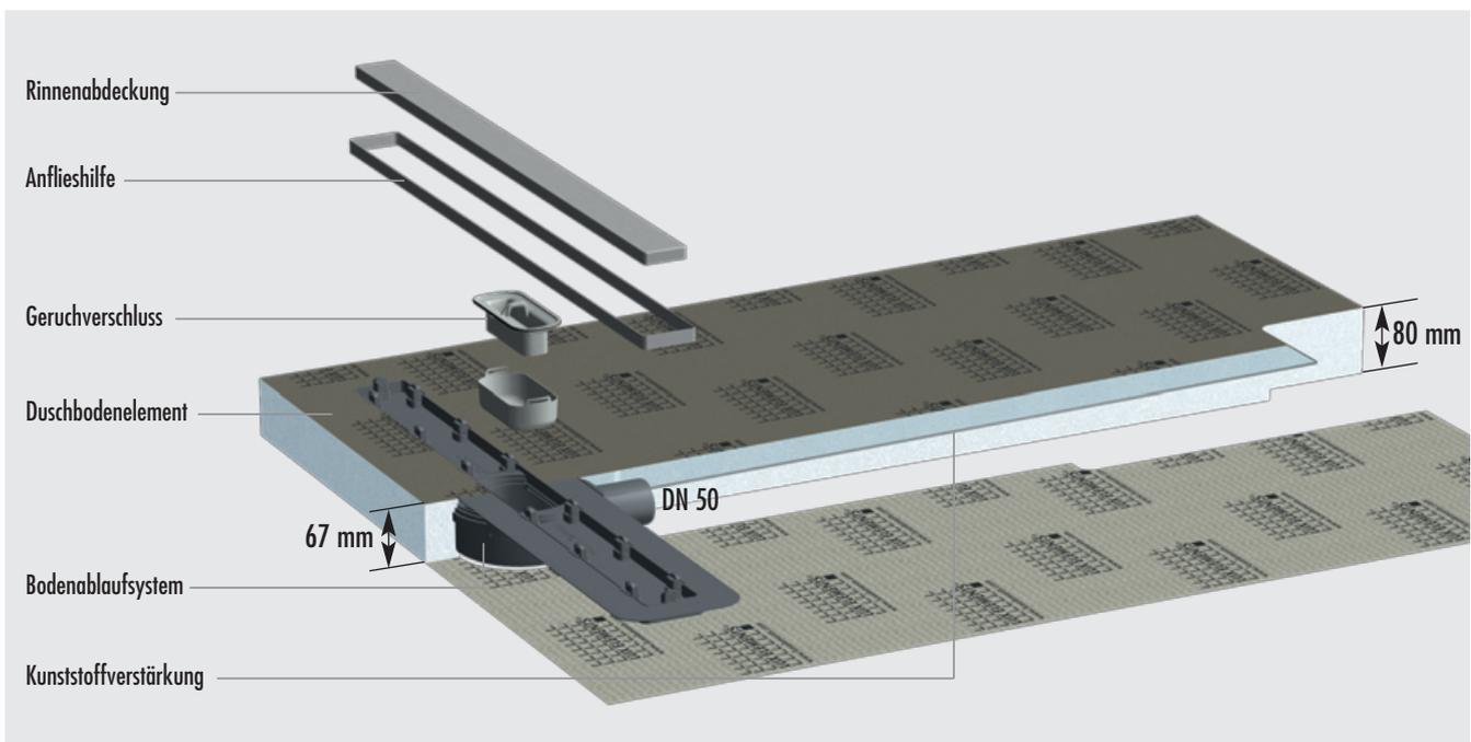
■ PRODUKTDATEN – LUX ELEMENTS®-TUB-LINE COMBI
