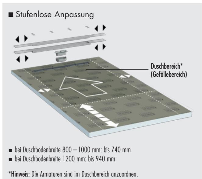
■ PRODUKTDATEN – LUX ELEMENTS®-TUB-LINE BOL V
